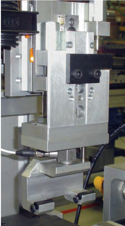
Assembly force monitoring using 208C Series force sensor
