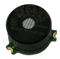
The compensator is made in the same way as a detector device except that instead of incorporating a catalyst in the coating layer, the device is treated so that oxidation cannot take place.
